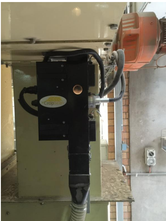
Figure 6. NIR In Line Analyser installed in an Australian flour mill
